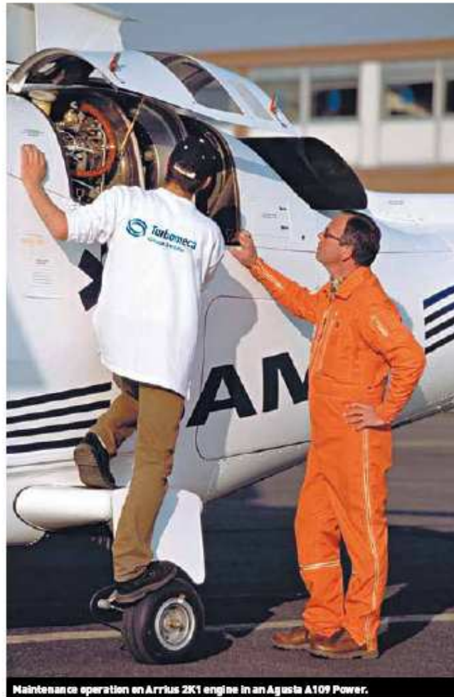
Maintenance operation on Arrius 2K1 engine in an Agusta A109 Power.
